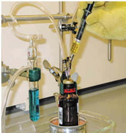
A recommended set-up for syringing tert-butyllithium includes inert gas supply and venting to a bubbler, as well as a glass syringe. <http://cen.acs.org>
