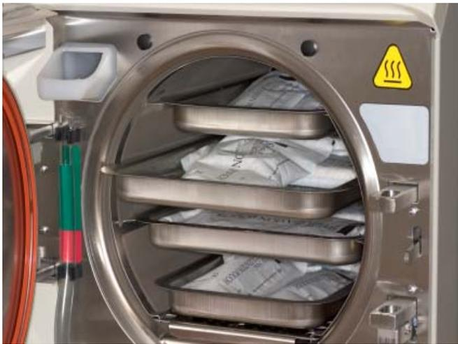
Autoclave bags in pans—not contacting the walls of the autoclave.
